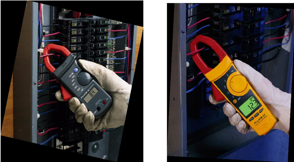
Figure 1. One current—two readings. Which do you trust? The branch circuit above feeds a non-linear load with distorted current. The true-rms clamp reads correctly but the average responding clamp reads low by 32 percent.
