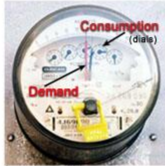
Commercial Electric Meter
